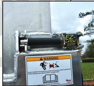
E-Z latch with oval-shaped stop/turn/tail light
